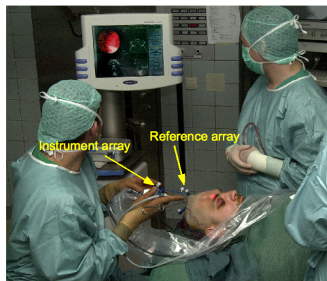
Fig. 10. Tracking of a surgical screw driver through an instrument array. Image is courtesy of Jürgen Hoffmann, Universität Tübingen.
