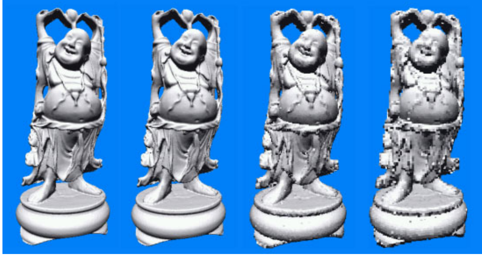
Figure 11: The Happy Buddha rendered by the z-buffer algorithm (leftmost) and by our approach with different splat sizes: From left to right: splat size 1, 3 and 5.
