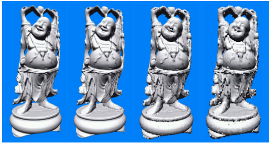
Figure 6: The Happy Buddha rendered by the z-buffer algorithm (leftmost) and by our approach with different splat sizes: From left to right: splat size 1, 3 and 5. (This figure is reproduced in color on page 000.)
