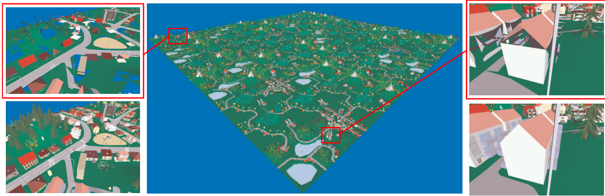
Figure 12: Two parts of the image are zoomed and show that only samples of polygons are rendered. Below, the corresponding parts of the original scene are rendered by the z-buffer algorithm. We used splat size 4 and left out the precomputation of color values for better illustration. (This figure is reproduced in color on page 000.)
